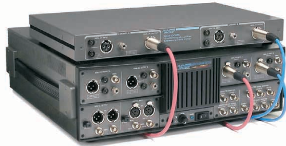
Audio Precision Cascade Plus instrument with AUX-0025 signal conditioning pre-filter.
